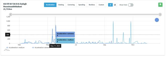
**The Violations Dashboard** analyzes violations for drivers, vehicles, or groups, presenting violation scores on a line chart for each type (**Acceleration**, **Braking**, **Cornering**, **Speeding**, **Reckless**) with configurable levels (e.g., medium, extreme). Integrated with **Track3**, the definition of an extreme violation is configured within Track3.
