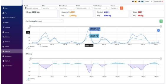
Vital for fleet management, offering a **comprehensive** view of fuel efficiency. Displays total mileage, actual fuel consumption, and calculates **CO2** emissions, based on fuel type. Assists in assessing the fleet's ecological footprint. Compares '**Consumed'** (actual) with '**Nominal'** (expected) values.
