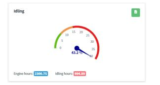
**Idling:** Highlights the total engine hours and calculates the percentage of idling engine hours against the total engine hours.
